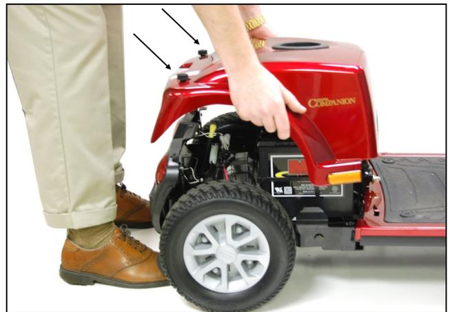
FIGURE 16. REMOVING THE REAR SHROUD
