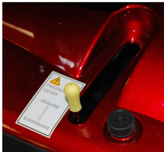
FIGURE 12. FREEWHEEL LEVER (DISENGAGED)
