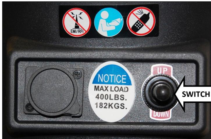
FIGURE 10. POWER ELEVATING SEAT SWITCH
