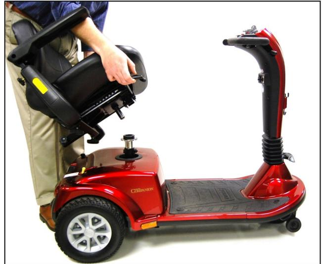
FIGURE 15. REMOVING THE SEAT
