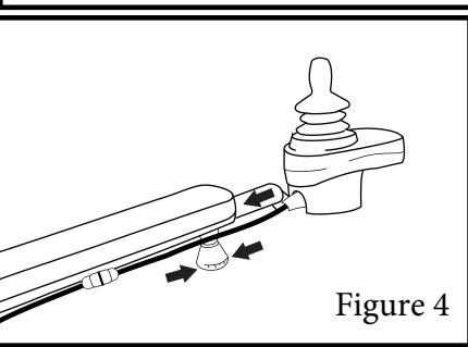
**Step 5.** Press the latch for one of the anti-tip brackets, which are located at the inside of the rear wheels under the motors. Fully extend the anti-tip until it locks into place. See figure 5. Repeat step 5 for the opposite anti-tip.
