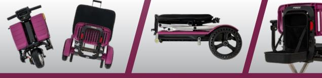
Disassembles into two pieces with the heaviest piece weighing 32.8 lbs.
