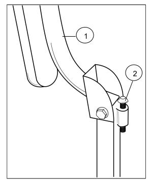
Figure 6. Armrest Width Adjustment
