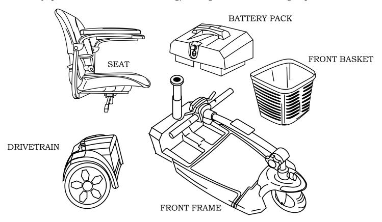
Figure 19. Buzzaround Lite™ Components (Model GB107)
