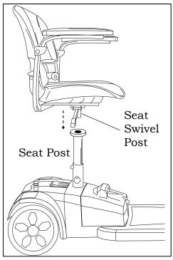
Figure 24. Installing the Seat
