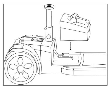
Figure 22. Battery Pack Installation
