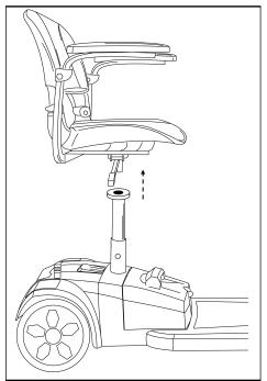
Figure 15. Removing the Seat
