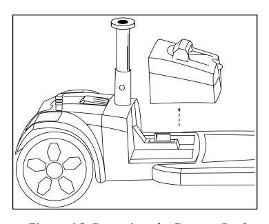
Figure 16. Removing the Battery Pack
