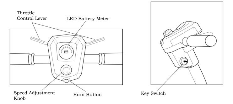
Figure 5. Buzzaround Lite<sup>TM</sup> Tiller Control Panel
