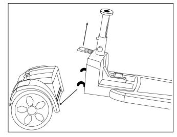
Figure 21. Connecting Frame and Drivetrain
