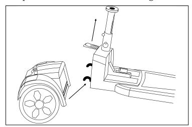
Figure 18. Separating the Drivetrain and Frame
