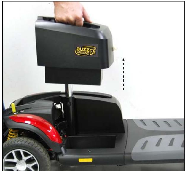
**Figure 15. Removing the Battery Pack**
