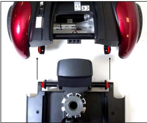
**Figure 19. Drivetrain Alignment**
