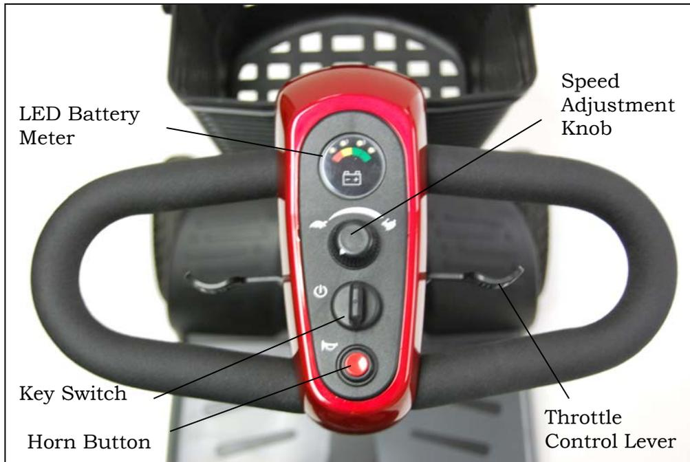
**Figure 5. Buzzaround Extreme™ Delta Tiller Control Panel**
