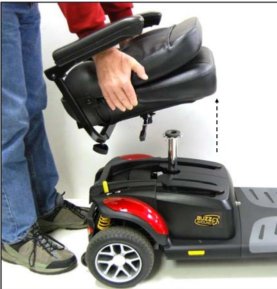
**Figure 14. Removing the Seat**
