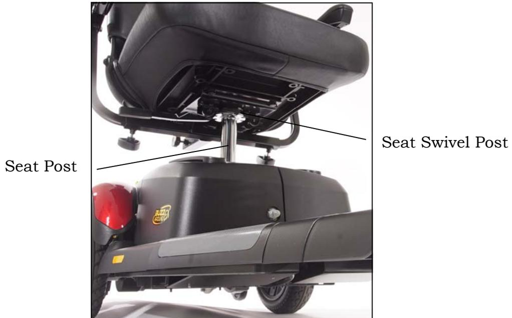
**Figure 23. Installing the Seat**
