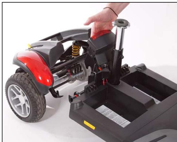
**Figure 17. Separating the Drivetrain and Frame**
