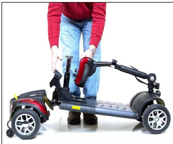
**Figure 20. Connecting Frame and Drivetrain**
