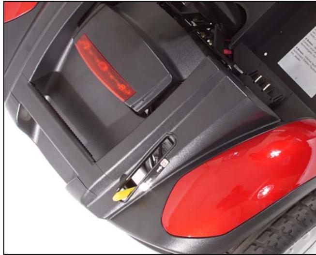
**Figure 11: Freewheel Lever (Drive Position)**
