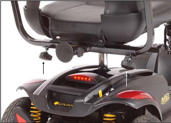
**Figure 6. Armrest Width Adjustment**
