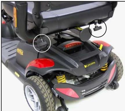
**Figure 8. Armrest Width Adjustment**
