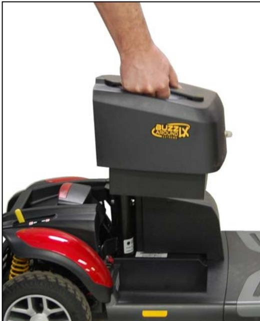
**Figure 23. Battery Pack Installation**
