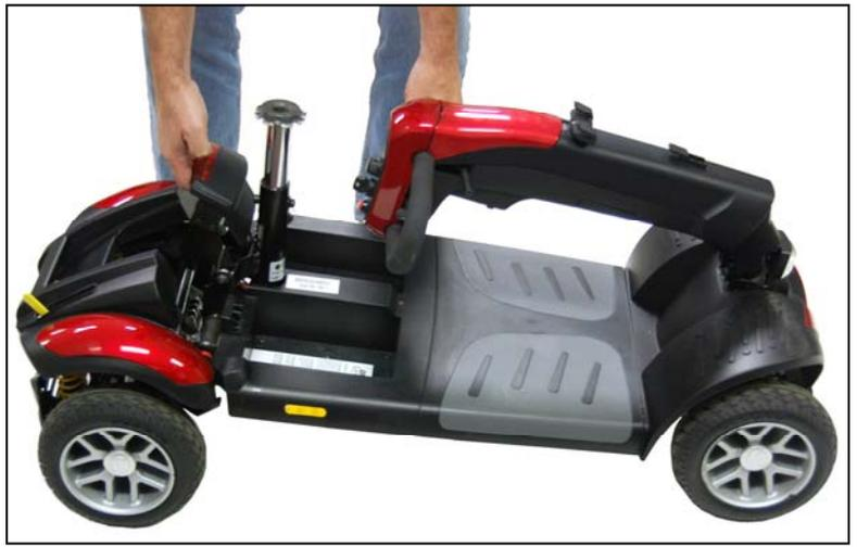
**Figure 22. Connecting Frame and Drivetrain**
