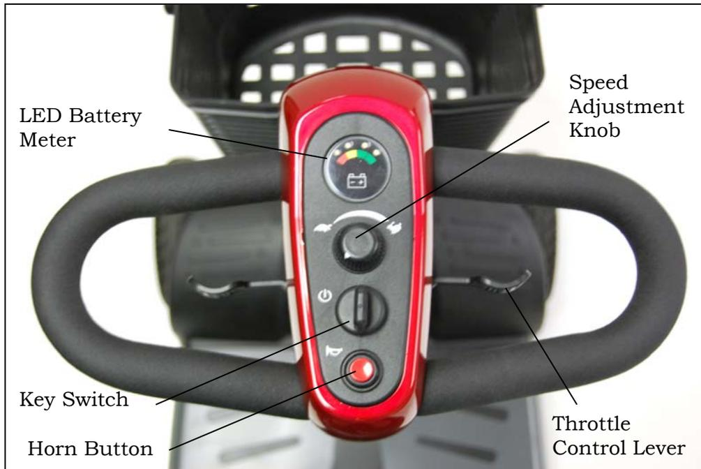
**Figure 5. Buzzaround Luxury™ Delta Tiller Control Panel**
