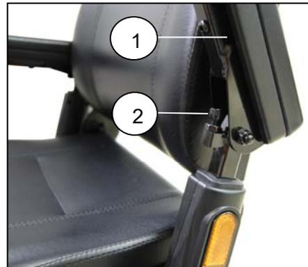
**Figure 9. Armrest Angle Adjustment**
