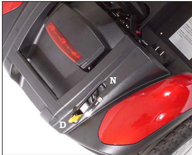
**Figure 13: Freewheel Lever (Drive Position)**
