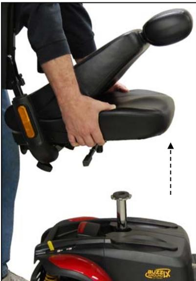
*Figure 16. Removing the Seat*
