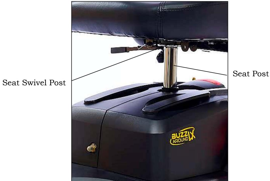
**Figure 25. Installing the Seat**
