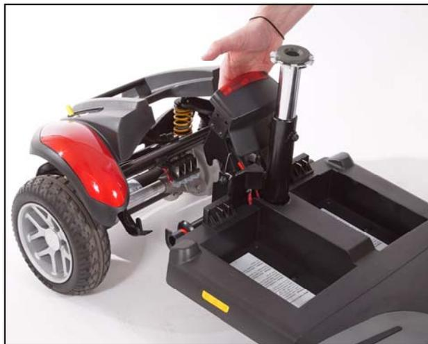
**Figure 19. Separating the Drivetrain and Frame**
