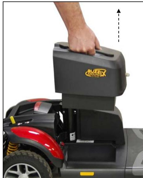
*Figure 17. Removing the Battery Pack*
