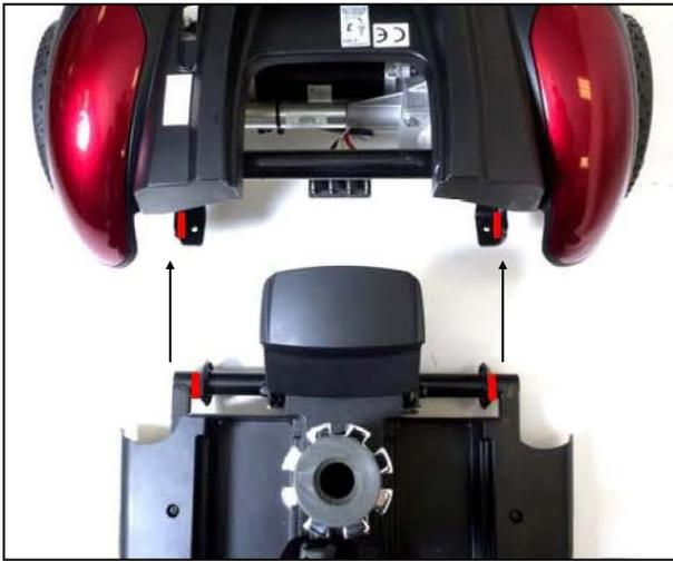
**Figure 21. Drivetrain Alignment**
