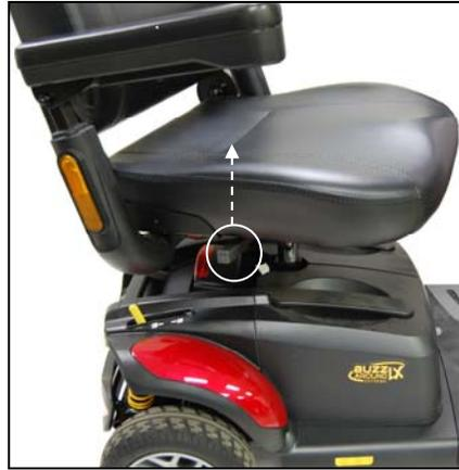
**Figure 10: Seat Rotation Adjustment**
