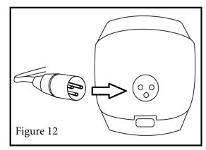
WARNING Failure to align and/or insert the plug in the correct orientation may damage the controller and render your power wheelchair non-operational.
