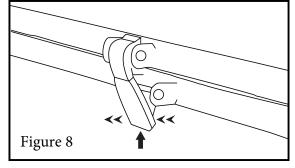
WARNING The two anti-tip brackets must be fully extended and locked to allow the power wheelchair to stand while in the folded position. Failure to comply will cause the power wheelchair to tip and fall over. This may result in serious injury to you and others near you.
