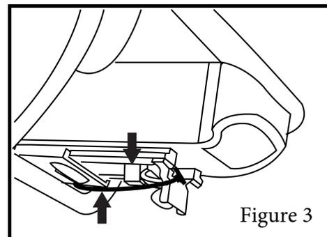
2. Remove the zip tie and block from the latch on the battery pack shown in figure 3.
