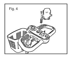
To install the cup holder, insert the cup holder within the basket and run the provided screws through the cup holder, basket and backing plate. Apply the washers and the Nyloc nuts to the screws and tighten. See figure 5.
