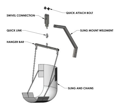
2. To install the sling seat, first remove the existing chair from the Mighty lift by removing the two (2) 5/16" bolts, washers and nylocks and sliding the chair and chair cradle off of the top casing.
