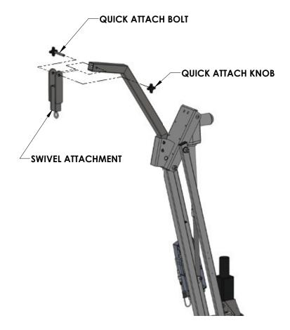
5. Install the hanger bar and sling onto the swivel attachment using the supplied quick link. Once the assembly is complete, adjust the chains to best fit the user and/or the pool area.
