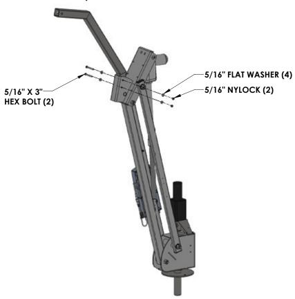
4. Install the swivel attachment onto the sling mount weldment using the supplied quick attach bolt and knobs.
